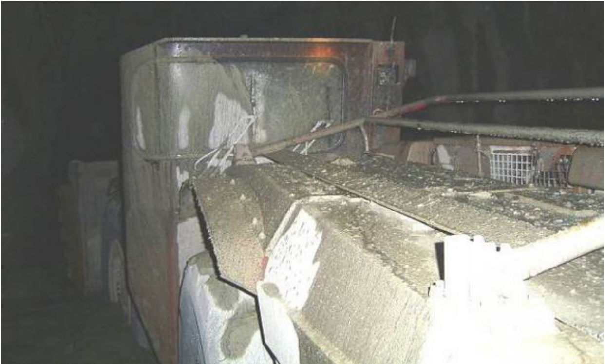
Photograph 2: Rear view of the bogger that was pushed down the drive below VR5A shaft. The mud material coated the bogger up to the cabin level. Photograph courtesy of Cadia East mine.
