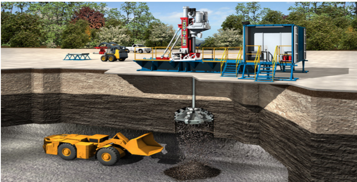
Picture 1: Representational view of the reaming process. Illustration only. Does not depict mine's actual bogging procedure.
