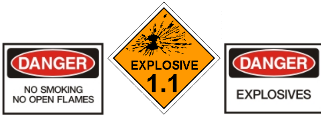
Figure 1: Signs to be marked: No Smoking sign, Explosive hazard class diamond, and Explosives sign.
