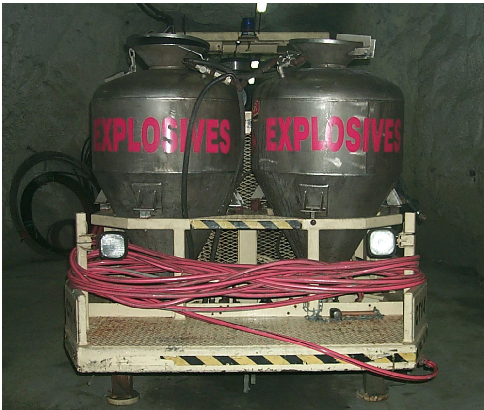
Figure 2: Charge car with kettles clearly labelled and blue flashing light mounted on drivers cabin
